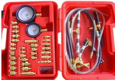
**KA-7237K Instructions For Multi-Port Fuel Injection Pressure Testing**
