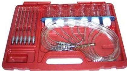
**KA-2898KQC Flow Meter common Rail Set ( Quick Replacement )**
