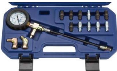
**KA-7421B Master Cylinder Pressure Test Kit (Brake & Clutch)**
