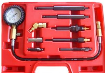
Easy-to-use compression tester is designed specifically for medium-duty engines equipped with glow plugs. Dual reading gauge measures compression to 1000 PSI and 7000 kPa. Gauge has a push-button release valve and quick disconnect fittings on the hose end. Tester comes with all the necessary glow plug and nozzle adapters in a handy storage case. Tester service these engines:
