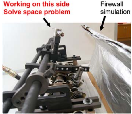
Manual working(for limited space because of firewall)
